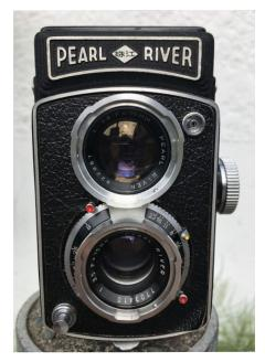
The Pearl River namesake of this camera flows through the Guangdong Delta. The Like the Eastar. the Pearl River uses 120 film for twelve 6x6 images (a 6x4.5 mask is available if one would prefer 16 images per roll). It has shutter speeds from 1/25 to 1/250. It has no Bulb mode.
